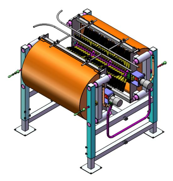
The Berry Wing Picker B-WP-3-48 is designed to clean the wings by the rotating rubber fingers which are placed to gently brush away cuticle matter, then rinse the matter away with use of the water spray nozzles. The model B-WP-3-48 is constructed of stainless steel, teflon, and aluminum for durability and easy clean up and has the capacity to process up to 300 birds per minute. The model B-WP-3-48 should be positioned after the last bird picker on the picking line.
